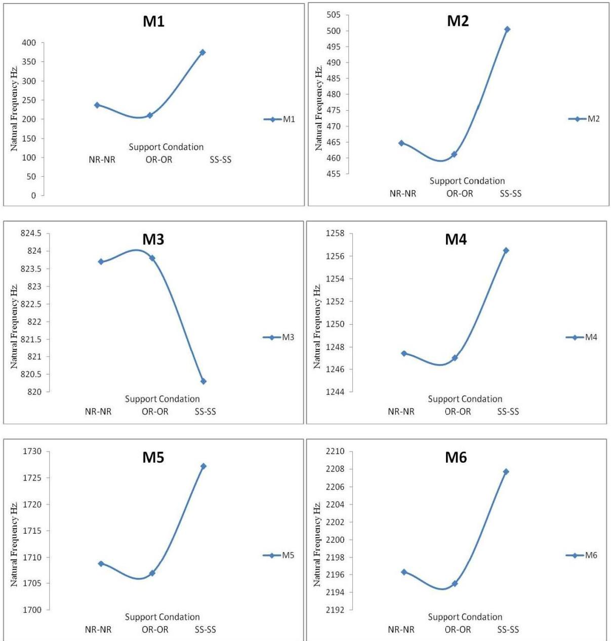
**Figure 4.** First six natural frequencies with different support conditions
