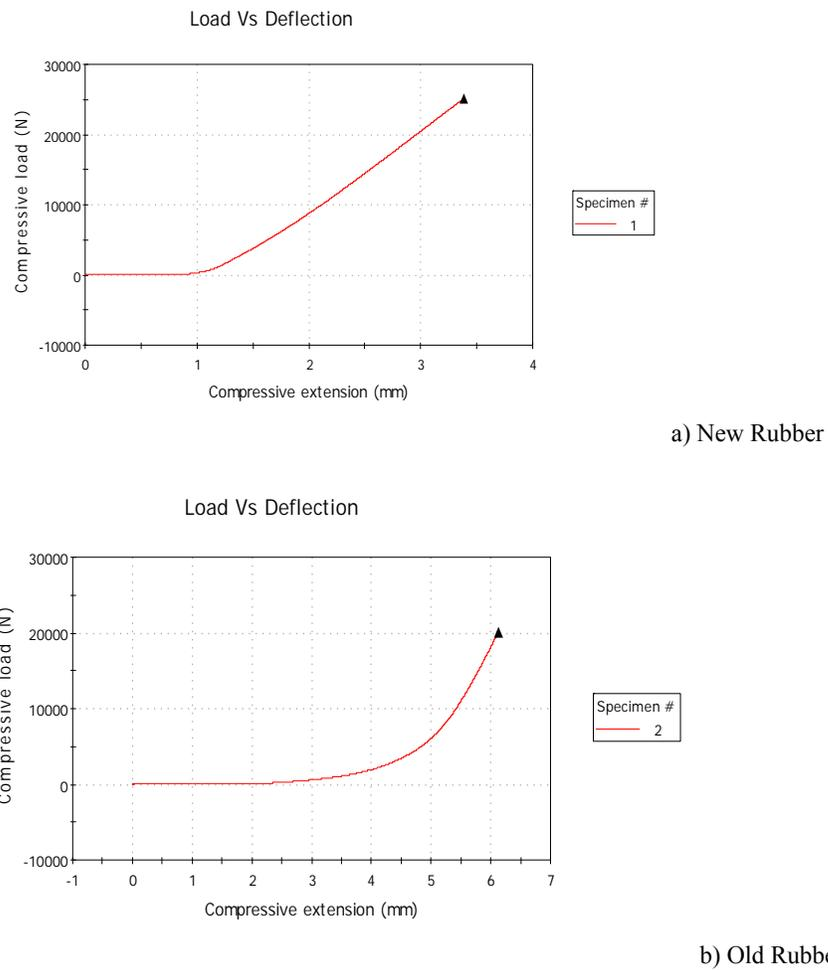
**Figure 3.** Load vs compressive extension curves for both rubber types.
