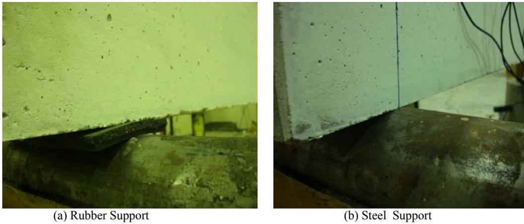
**Figure 2.** Different support conditions
