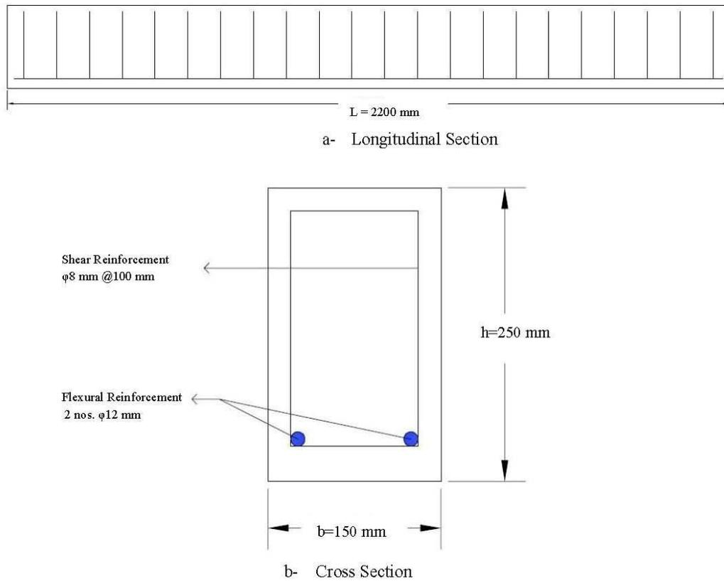
**Figure 1.** Details and dimensions of a Reinforced concrete beam.
