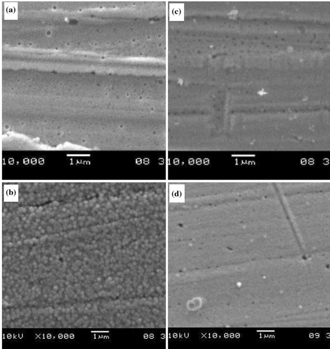
Fig. 7—SEM micrograph (magnification 10,000 times) of Ni-Co-Fe-Zn electrodepositon without PPMF: (a)  $-1.10$  V and (b)  $-1.30$ ; and with PPMF (9 T): (c)  $-1.10$  V, (d)  $-1.30$  V vs SCE.
