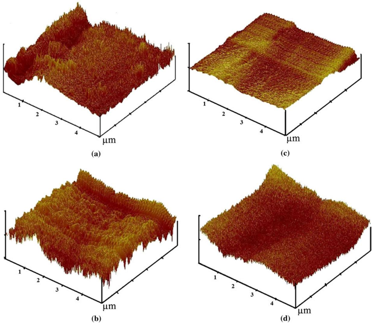
Fig. 9—AFM images of Ni-Co-Fe-Zn alloy surface electrodeposited in the absence of PPMF: (a)  $-1.10$  V and (b)  $-1.30$  V; and with PPMF (9 T): (c)  $-1.10$  V and (d)  $-1.30$  V vs SCE.
