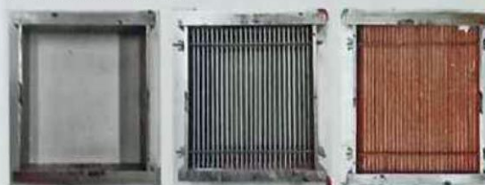
Figure 1. (a) Smooth channel, (b) Fin heat exchanger, (c) Fin metal foam heat exchanger
