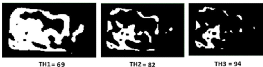
Fig. 2 Images were thresholded + 15% from the global threshold value (69, 82: global threshold value and 94) and binarised in the CTAnalyser software
