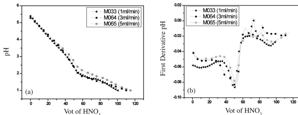
FIGURE 4. Titration curve and derivative of 0.10M AHM with 1.0 M HNO<sub>3</sub> at different rate of addition for (a) pH and (b) pH first derivative
