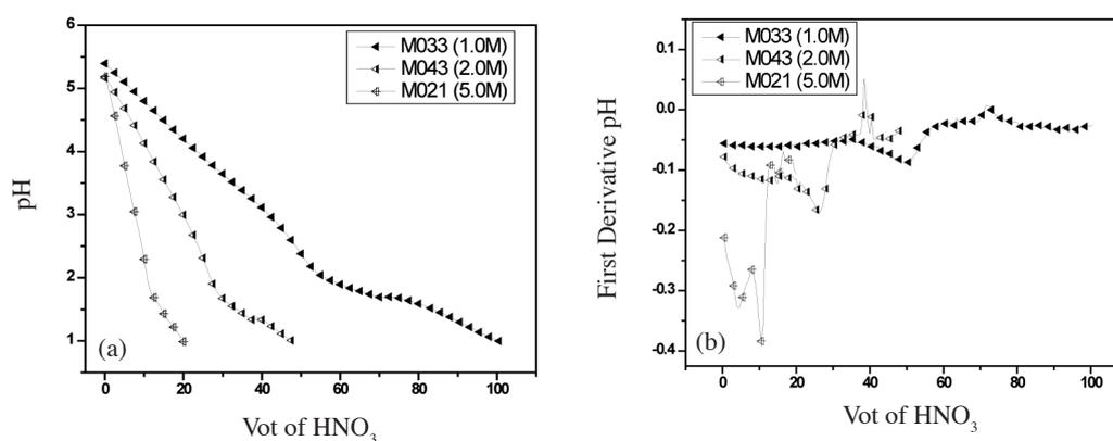
FIGURE 5. Titration of 0.10 M AHM with HNO<sub>3</sub> at different concentration for (a) pH and (b) pH first derivative
