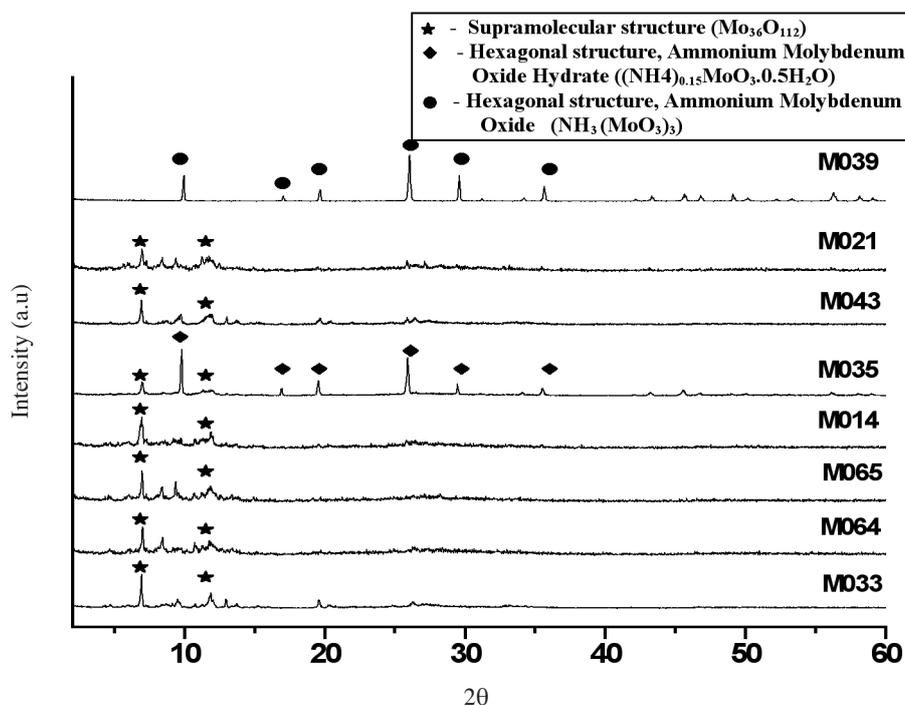
FIGURE 1. XRD patterns of synthesized samples
