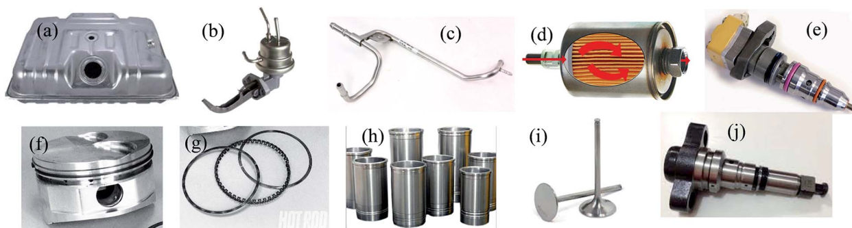
Fig. 7 Automotive components in engine and fuel systems: (a) fuel tank, (b) fuel pump, (c) fuel line, (d) fuel filter, (e) fuel injector, (f) piston, (g) piston ring, (h) cylinder liner, (i) valve, and (j) fuel filter plunger. Adopted from: http://www.certifiedmastertech.com/wordpress/2011/08/08/automotive-fuel-tank-problems/ , http://www.ebay.com/itm/Metal-Fuel-Line-09-10-VW-Jetta-Golf-MK5-TDI-CBEA-Diesel-03L-201-360-F-/351165118882 , http://www.agcoauto.com/content/news/p2_articleid/219 , http://dieseliq.com/common-reasons-diesel-fuel-injectors-fail , http://www.hotrod.com/how-to/engine/hrdp-9808-piston-ring-science/ , http://www.hotrod.com/how-to/engine/hrdp-9808-piston-ring-science/ , http://rajkot.all.biz/cylinder-liner-sleeves-g264983#.V06yPmh97b0 , http://www.dealernews.com/dealernews/article/honda%E2%80%99s-crf450r-gets-engine-makeover-pro-circuit , http://boschnozzle.blog.163.com/blog/static/18481836020113222451735/ .
