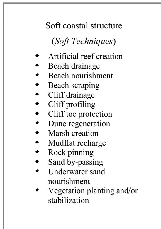
Figure 2: Soft coastal structures
