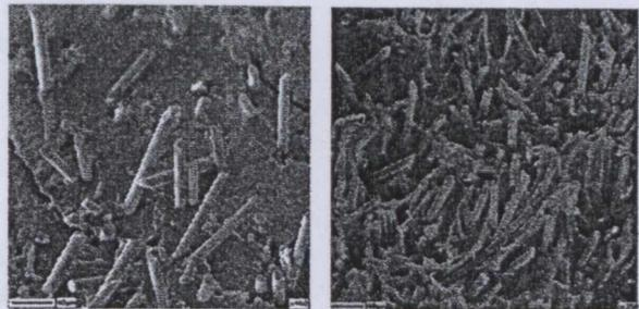
Fig. 8. SEM micrograph taken from tensile fracture surface of composite under dry (left) and wet (right) conditions.
