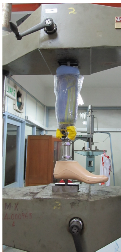
Figure 5 | Mechanical testing. Tensile testing for the new prosthesis coupling system.
