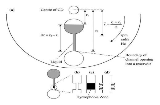
Fig. 1 a The microfluidic CD with hydrophilic capillary valve, b hydrophobic valve with constriction, c hydrophobic valve with hydrophobic zone in an otherwise hydrophilic channel, d fishbone valve
