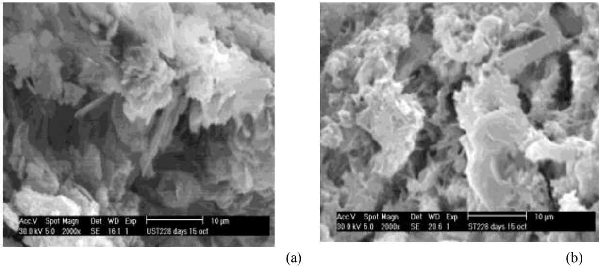
**Figure 4:** Scanning electron micrograph of a) original peat soil b) stabilized peat
