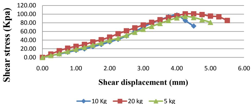
**Figure 3:** Shear stress of stabilised peat for different normal load condition from direct shear box test
