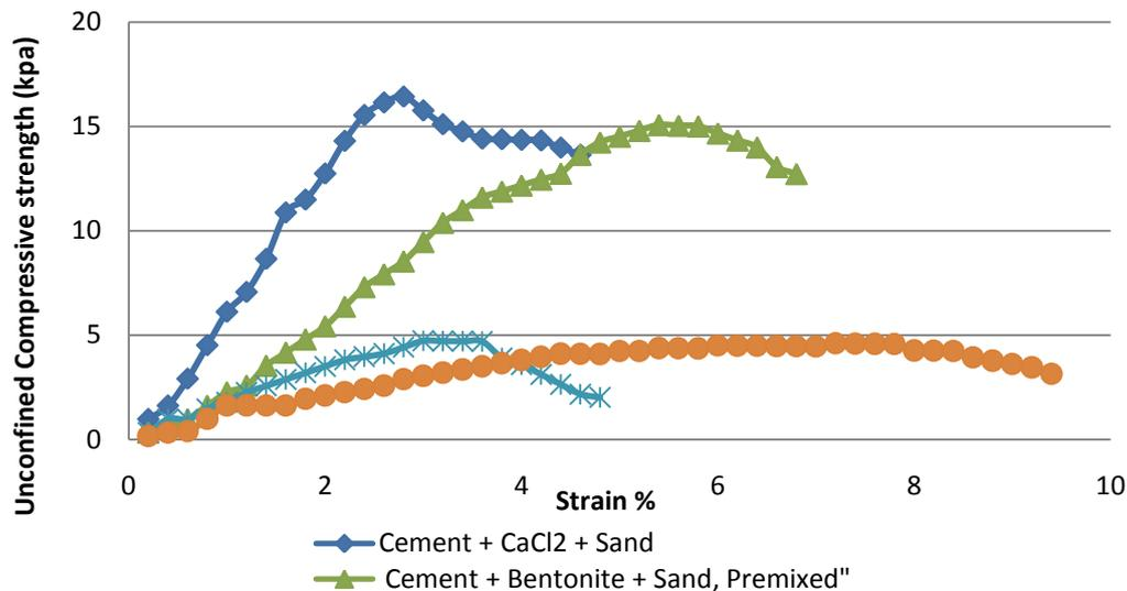
**Figure 2:** Unconfined compressive strength of collected sample from stabilised column.
