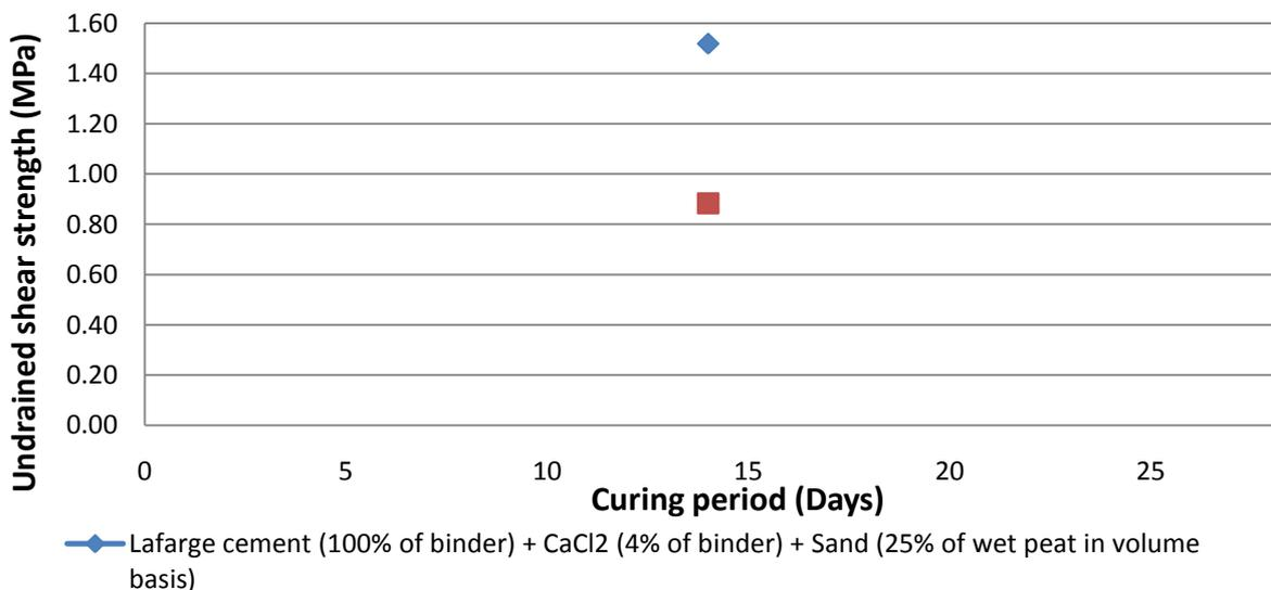
Figure 1: Undrained shear strength of stabilised column after 14 days curing time
