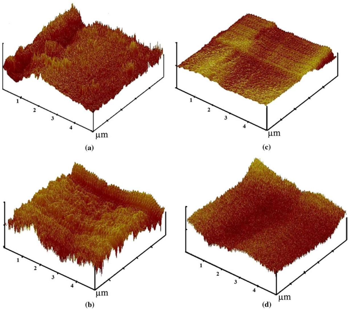
Fig. 9—AFM images of Ni-Co-Fe-Zn alloy surface electrodeposited in the absence of PPMF: (a)  $-1.10$  V and (b)  $-1.30$  V; and with PPMF (9 T): (c)  $-1.10$  V and (d)  $-1.30$  V vs SCE.
