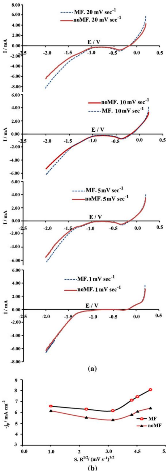
Fig. 2—(a) Voltammograms of Ni-Co-Fe-Zn alloys from EMIC/EG solution at various scan rates ( $1$  to  $20\text{ mV s}^{-1}$ ) in the presence and absence of the PPMF (9 T). Concentration of each element in solution was  $0.01\text{ M}$  during the process. (b) Plot of  $j_p$  vs  $SR^{1/2}$  taken at currents at  $-2\text{ V}$  vs SCE from the voltammograms in (a).
