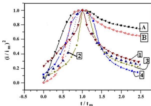
Fig. 4—The  $(i/i_m)^2$  vs  $t/t_m$  curves for deposition of the Ni-Co-Fe-Zn alloys from EMIC/EG solution at different current densities in the absence and presence of a PPMF: (a) instantaneous, (b) progressive, and the electrodeposited layers: (1) at  $-1.10$  V (without PPMF), (2) at  $-1.10$  V (with PPMF), (3) at  $-1.30$  V (without PPMF), and (4) at  $-1.30$  V (with PPMF) vs SCE.
