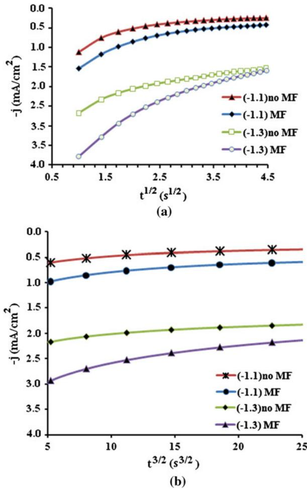
Fig. 5—Plots of (a)  $i$  vs  $t^{1/2}$  and (b)  $i$  vs  $t^{3/2}$  from initial transients in Fig. 3 for the Ni-Co-Fe-Zn alloy deposition to show the instantaneous and progressive nucleation mechanisms, respectively.
