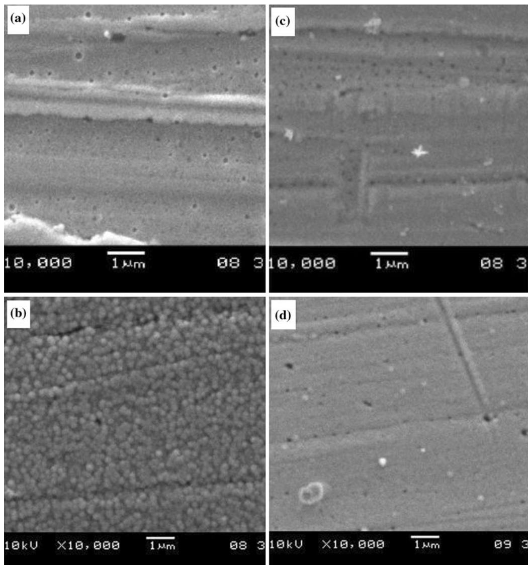
Fig. 7—SEM micrograph (magnification 10,000 times) of Ni-Co-Fe-Zn electrodeposition without PPMF: (a)  $-1.10\text{ V}$  and (b)  $-1.30\text{ V}$ ; and with PPMF (9 T): (c)  $-1.10\text{ V}$ , (d)  $-1.30\text{ V}$  vs SCE.
