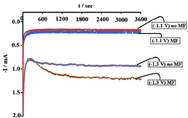
Fig. 3—Chronoamperometry of Ni-Co-Fe-Zn alloys in the presence and absence of the PPMF (9 T) at constant applied potentials ( $-1.10$  and  $-1.30\text{ V}$ ) from EMIC/EG bath. Current density values were enhanced with PPMF at the same potential.
