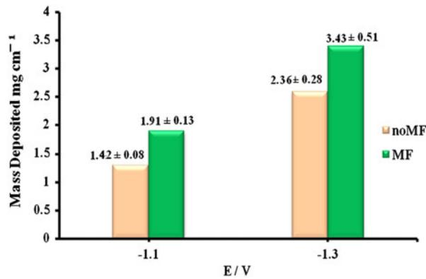
Fig. 6—Mass of deposited Ni-Co-Fe-Zn alloys is shown and increases with the increase in deposition potential with the presence and absence of the PPMF from EMIC/EG solvent.
