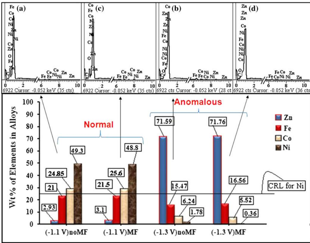
Fig. 8—EDX spectrum (top) and results (bottom) of the weight percentages of elements in Ni-Co-Fe-Zn alloys electrodeposited from EMIC/EG solvent at potentials of  $-1.10\text{ V}$  and  $-1.30\text{ V}$  with the absence and presence of the PPMF (9 T), together with the total percentages of the elements in all four electrodeposited alloys. The CRL line of Ni is 25 pct.
