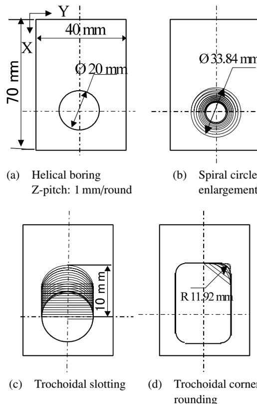
Fig. 9 Workpiece and tool paths used in each process
