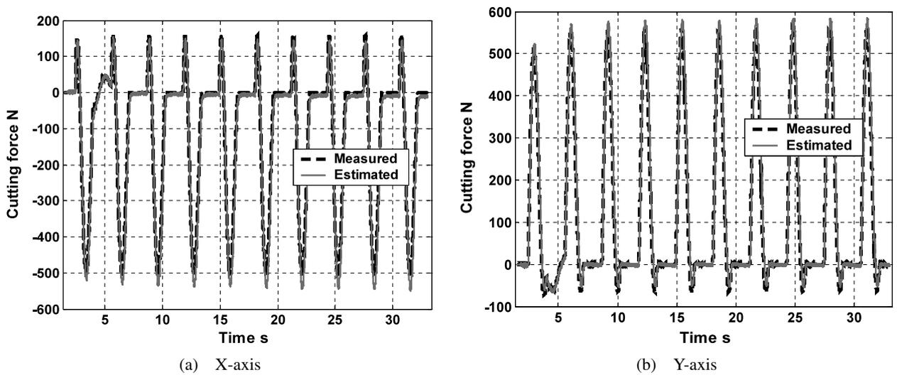
Fig. 12 Comparison of estimated and measured cutting forces in trochoidal-cut
