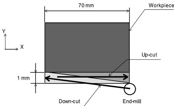
Fig. 6 Workpiece and tool paths
