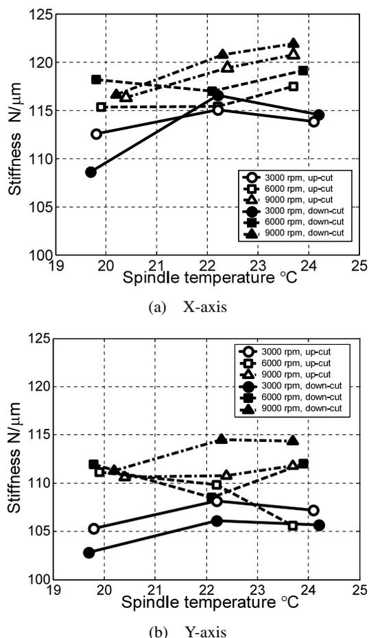
Fig. 8 Identified spindle stiffness in different cutting conditions
