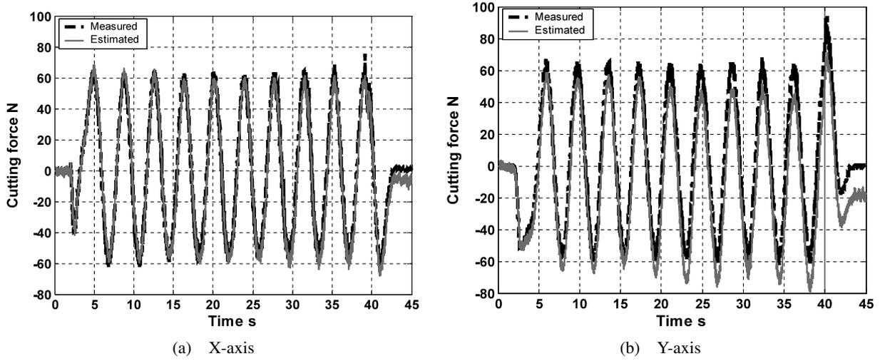
Fig. 10 Comparison of estimated and measured cutting forces in helical-cut
