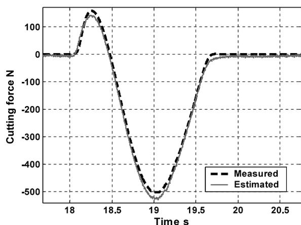
Fig. 15 Estimated and measured cutting forces in one cycle of trochoidal slotting process after the modification
