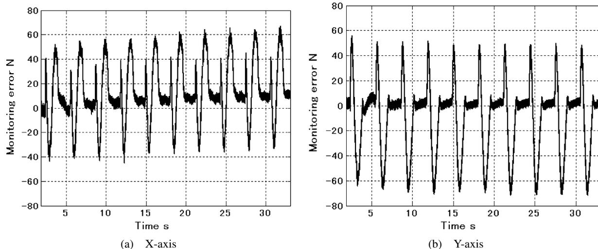
Fig. 13 Monitoring errors (measured minus estimated cutting forces) in trochoidal-cut
