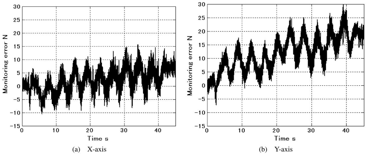
Fig. 11 Monitoring errors (measured minus estimated cutting forces) in helical-cut
