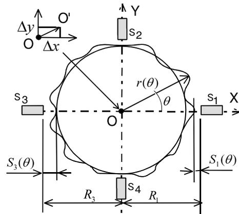
Fig. 2 The concept of the spindle displacement measurement
