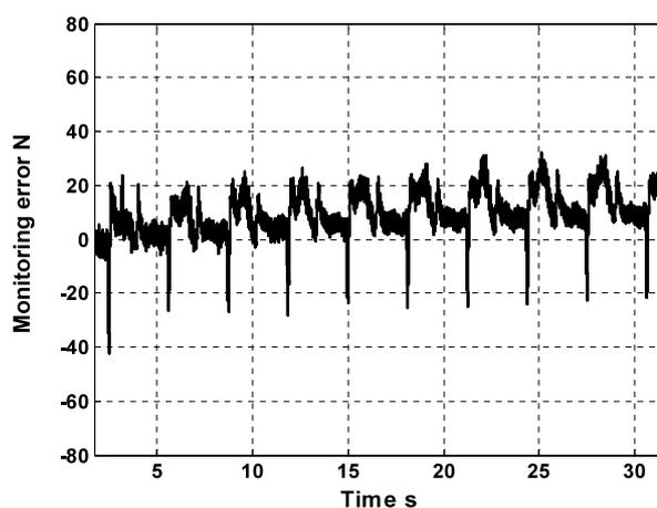
Fig. 16 Monitoring errors in the X-axis direction of trochoidal slotting process after the modification
