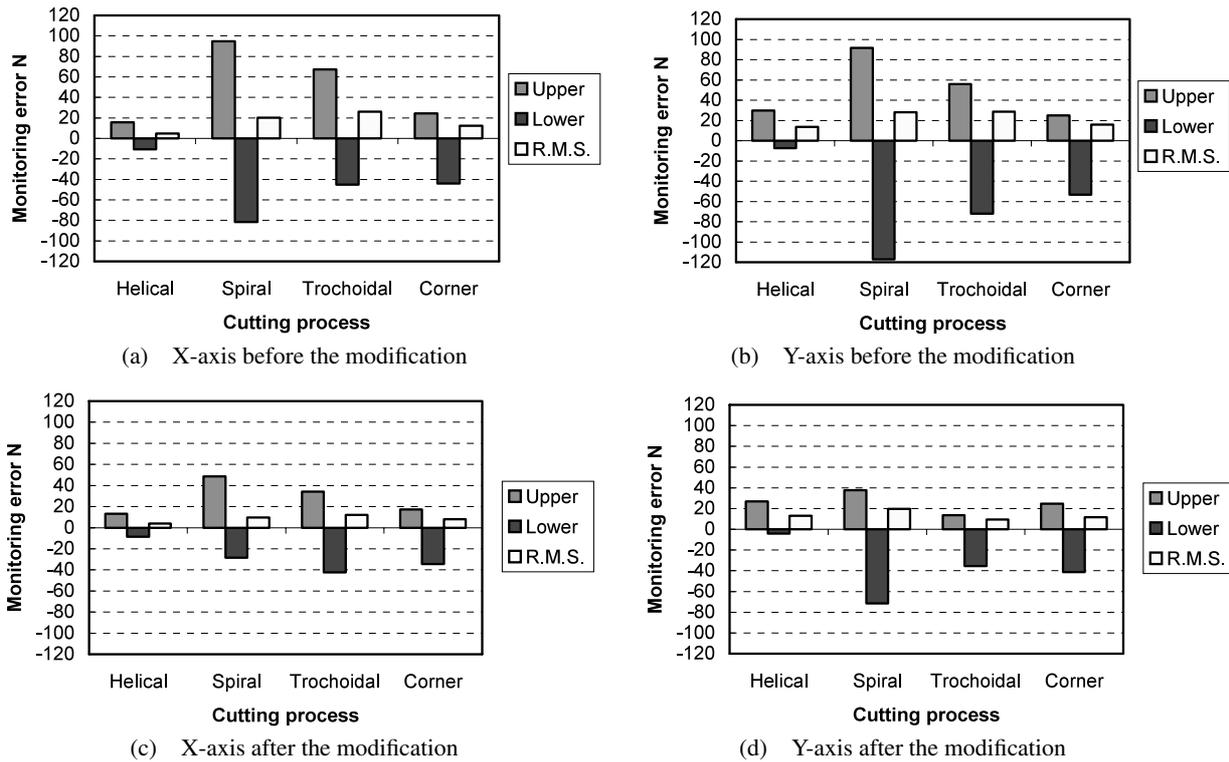
Fig. 17 The upper, lower and R.M.S. of the monitoring errors in each process before and after the modification
