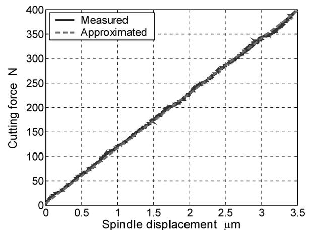
Fig. 7 An example of the relationships between the spindle displacement and the cutting force (direction: X-axis, spindle speed:  $3\,000\ \text{min}^{-1}$ , cutting mode: up-cut, spindle temperature:  $19.8^\circ\text{C}$ )
