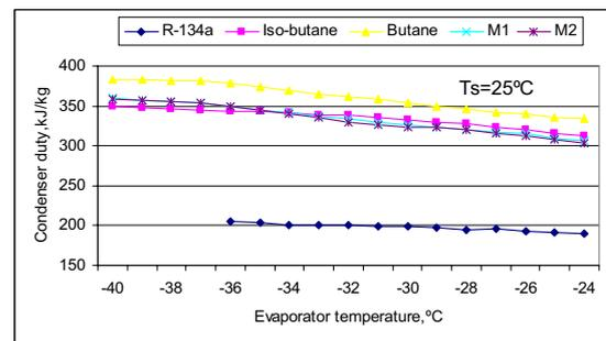
Figure 12 Effect of evaporator temperature on condenser duty at 25°C ambient temperature
