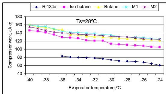
Figure 11 Effect of evaporator temperature on compressor work at 28°C ambient temperature
