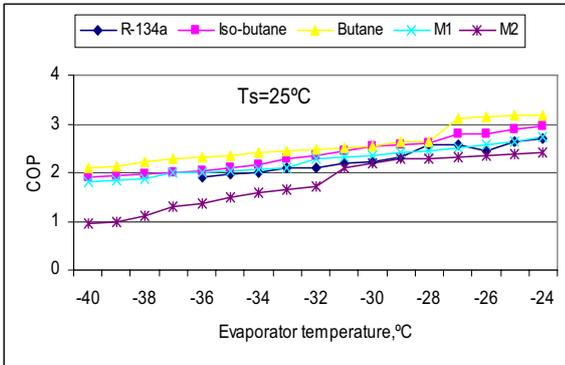
Figure 4 Effect of evaporator temperature on COP at 25°C ambient temperature
