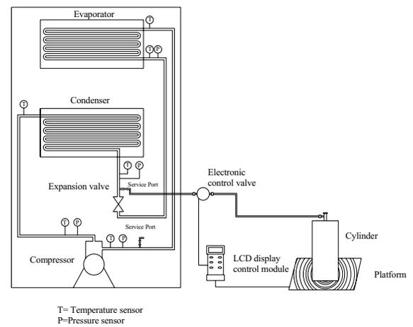
Figure 3 Schematic diagram of the charging system
