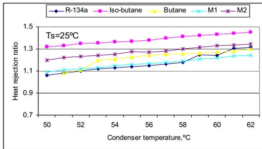
Figure 14 Effect of condenser temperature on heat rejection ratio at 25°C ambient temperature
