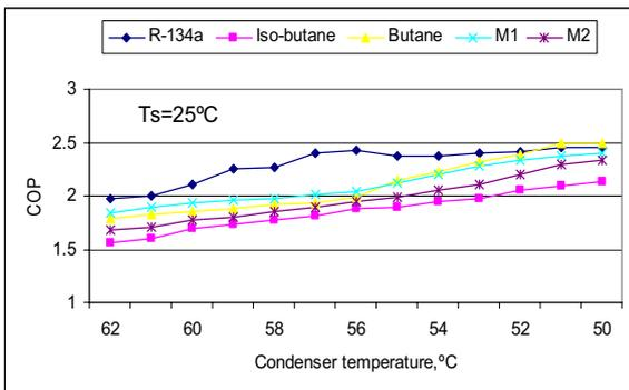
Figure 6 Effect of condenser temperature on COP at 25°C ambient temperature
