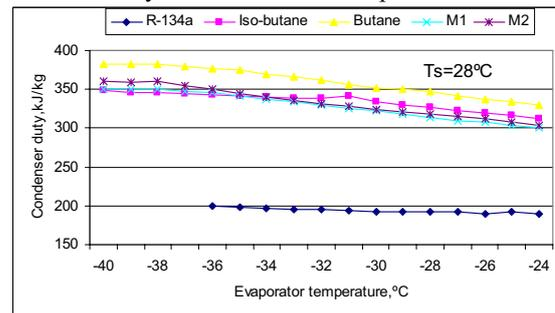
Figure 13 Effect of evaporator temperature on condenser duty at 28°C ambient temperature
