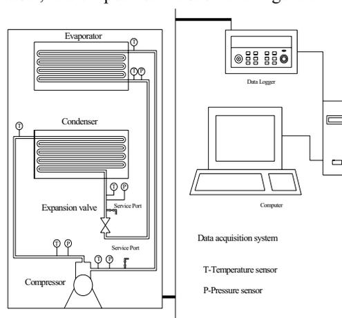
Figure 1 Schematic diagram of the test unit and apparatus
