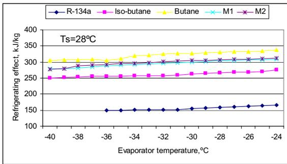
Figure 9 Effect of evaporator temperature on refrigerating effect at 28°C ambient temperature
