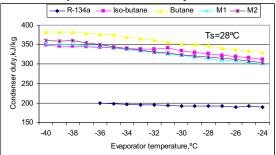
Figure 13 Effect of evaporator temperature on condenser duty at 28°C ambient temperature
