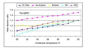
Figure 15 Effect of condenser temperature on heat rejection ratio at 28°C ambient temperature
