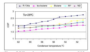
Figure 7 Effect of condenser temperature on COP at 28°C ambient temperature
