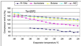
Figure 10 Effect of evaporator temperature on compressor work at 25°C ambient temperature
