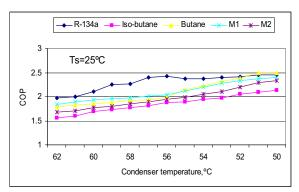
Figure 6 Effect of condenser temperature on COP at 25°C ambient temperature
