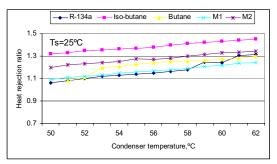
Figure 14 Effect of condenser temperature on heat rejection ratio at 25°C ambient temperature
