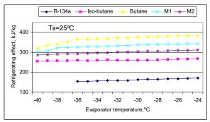
Figure 8 Effect of evaporator temperature on refrigerating effect at 25°C ambient temperature
