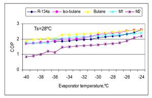
Figure 5 Effect of evaporator temperature on COP at 28°C ambient temperature
