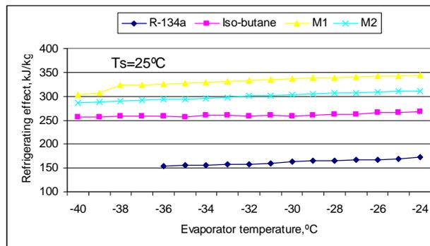
Figure 6 refrigerating effect versus inlet evaporator temperature
