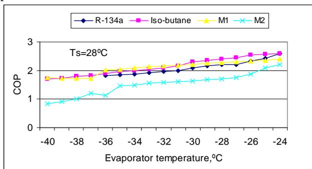
Figure 5 Effect of inlet refrigerant on co-efficient of performance
