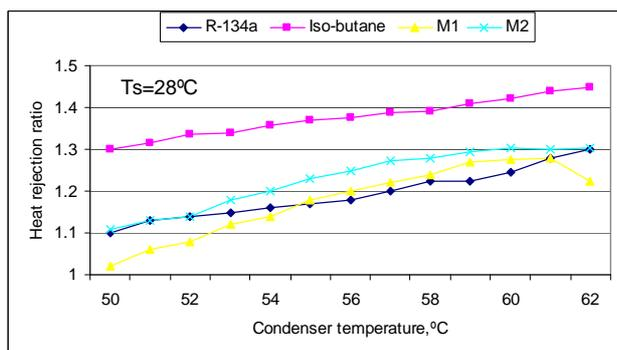
Figure 13 Heat rejection ratio at different condensing temperature
