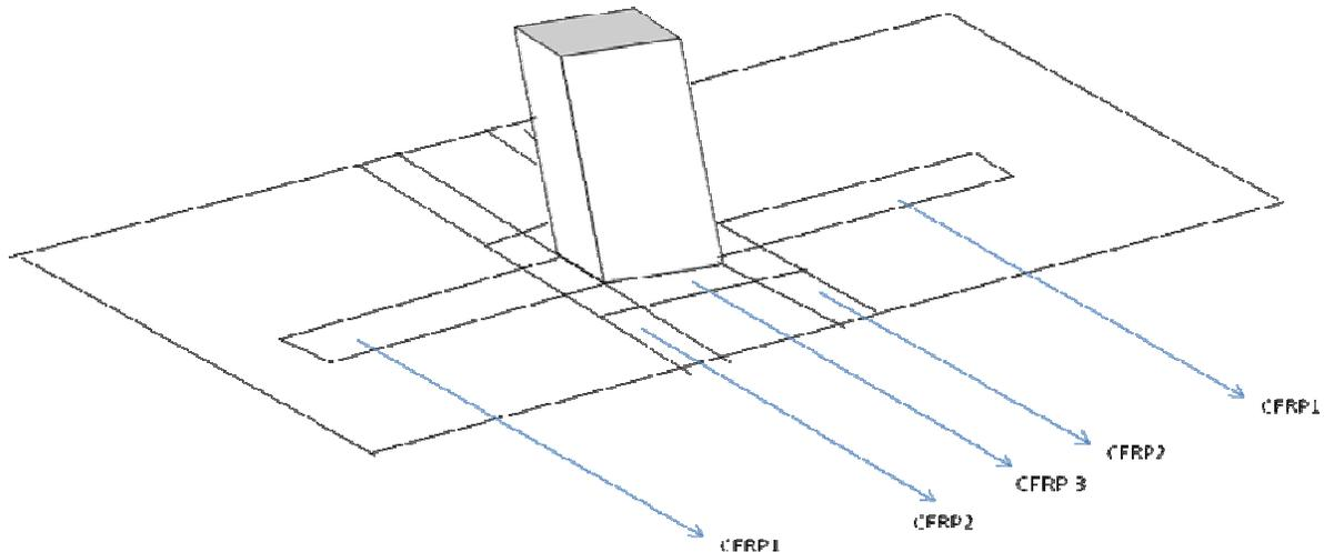
**Figure 1.** Method for applying CFRP in the negative moment region of continuous T beam.
