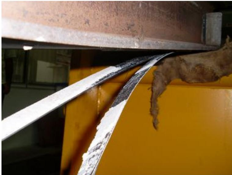
**Figure 9.** CFRP mid delaminating (splitting).
