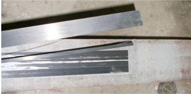
**Figure 8.** CFRP end delaminating (peeling).
