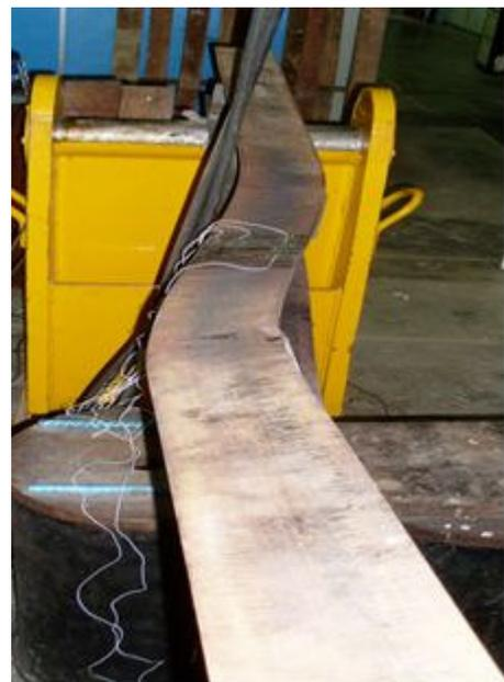
Figure 14. Lateral deformation (experiment).
