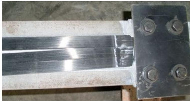
Figure 11. CFRP pulling out.
