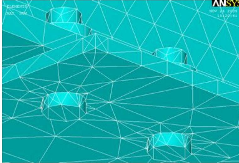
Figure 6. Meshing of end-anchor plate, obtained from ANSYS.
