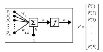
Figure 1. The neuron model with R-element in input.
