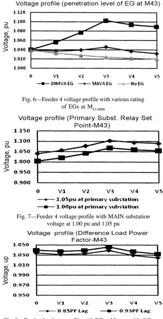
Fig. 8—Feeder 4 voltage profile with EG at  $\rm M_{43-MBB}$  with different network power factor
