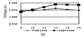
Fig. 4—Feeder 4 voltage profile with EG operating at: a) 0.85 leading power factor; and b) 0.85 lagging power factor
