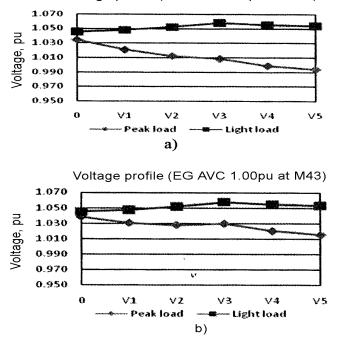
Fig. 5—Feeder 4 voltage profile with EG terminal voltage at: a) 1.00 pu; b) 1.03 pu
