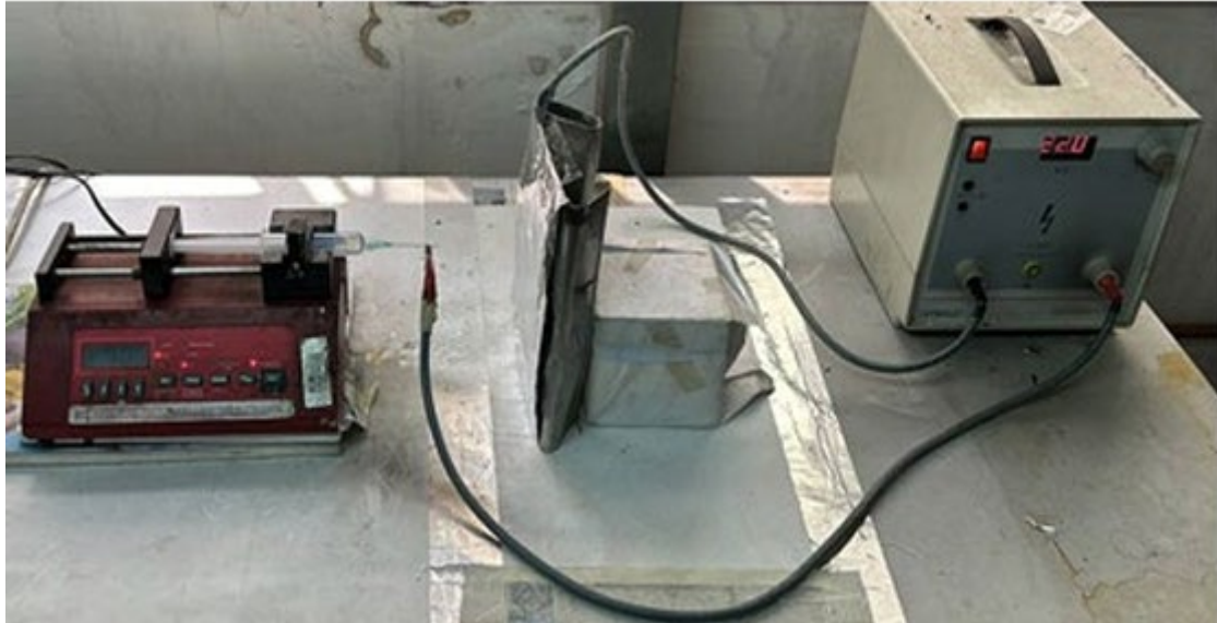
Figure 1. The electrospinning process setup.
