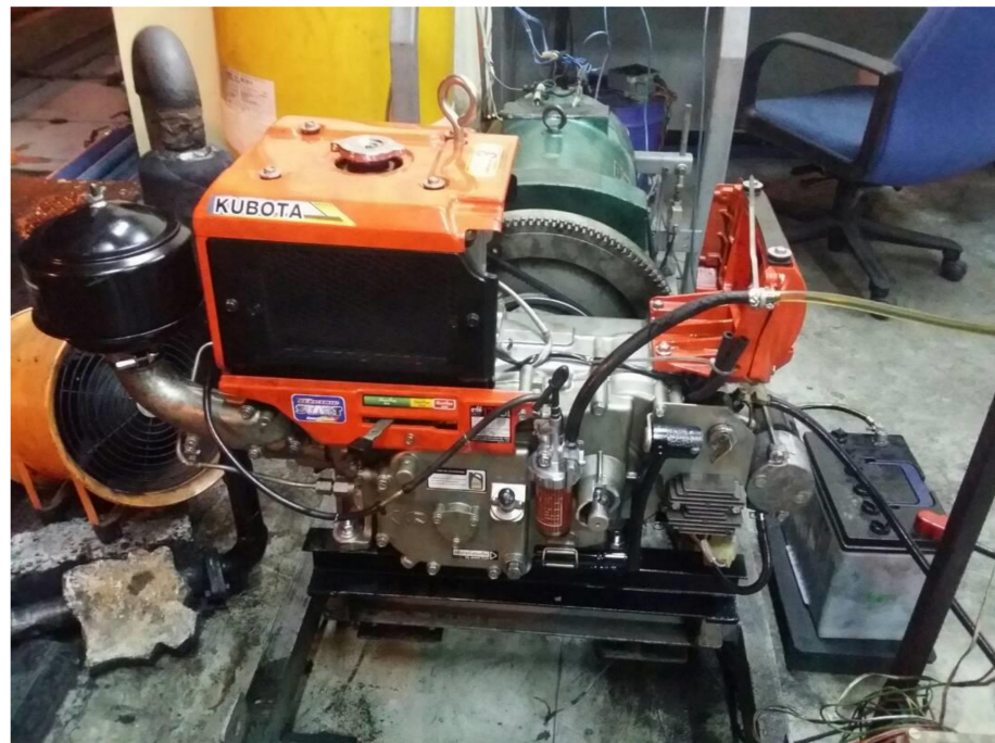
Figure 2. Kubota RT-125 diesel engine experimental setup.
