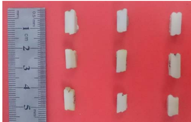
Figure 1: Layered specimens prepared from different shades of each restorative material.
