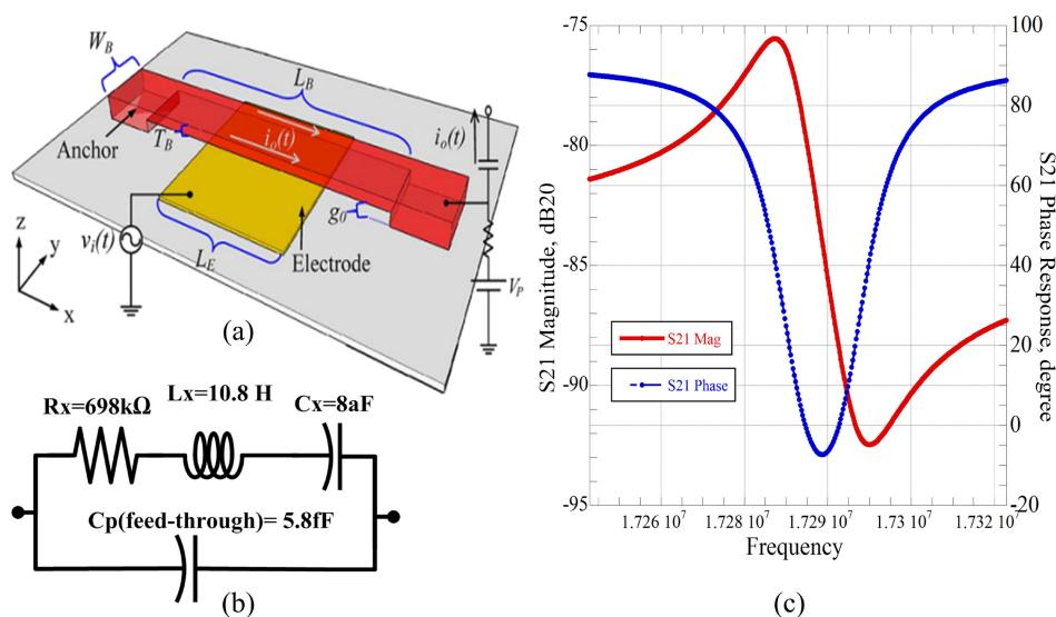
**Fig. 1.** (a) A 3D view of C-C beam MEMS resonator with necessary bias and signals (b) RLC equivalent model with electrically fitted lumped values of the MEMS (c) Insertion loss and phase shift response of it.
