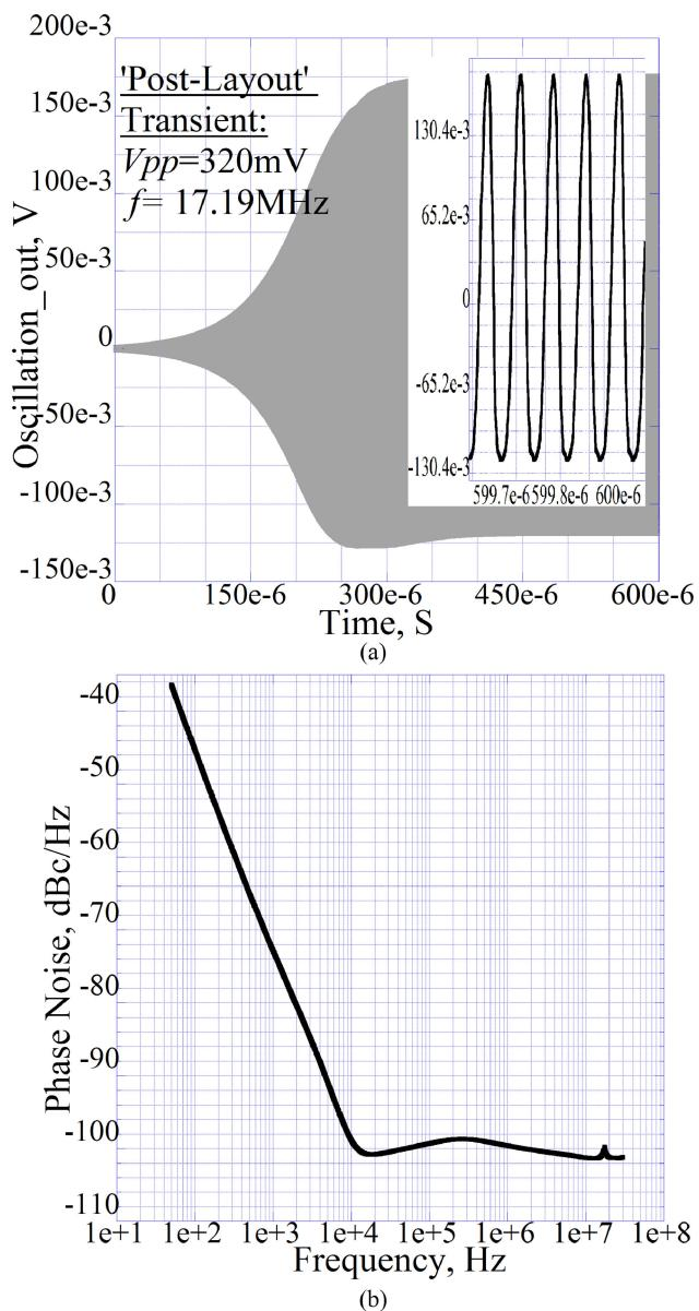
**Fig. 6.** (a) Oscillator output transient response (b) Oscillator phase noise response.
