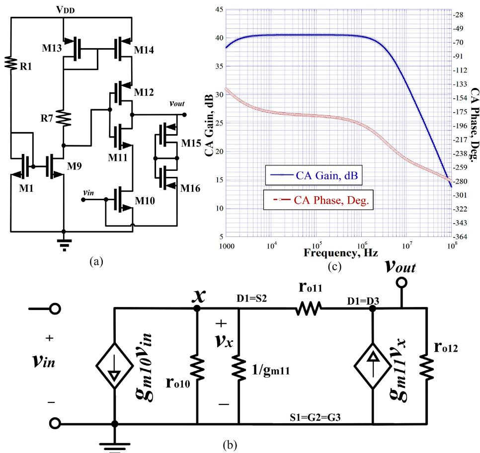
Fig. 4. (a) Cascode amplifier (b) Simplified small signal equivalent (c) Gain and phase response.
