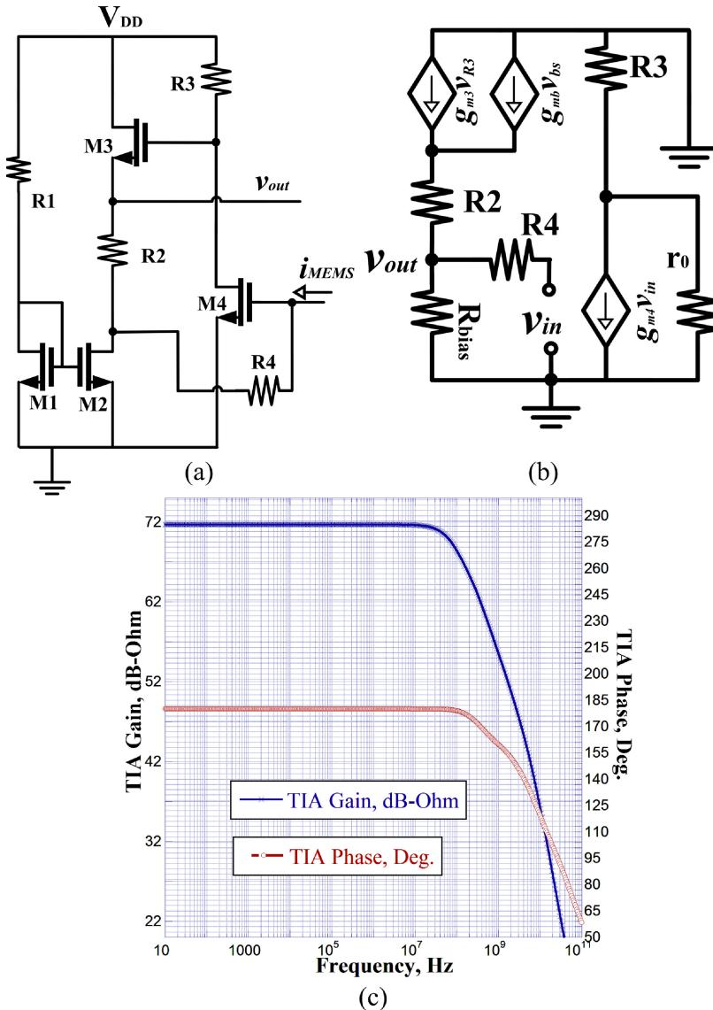
Fig. 2. (a) Schematic of transimpedance amplifier (b) Its small signal equivalent (c) TIA gain and phase response.
