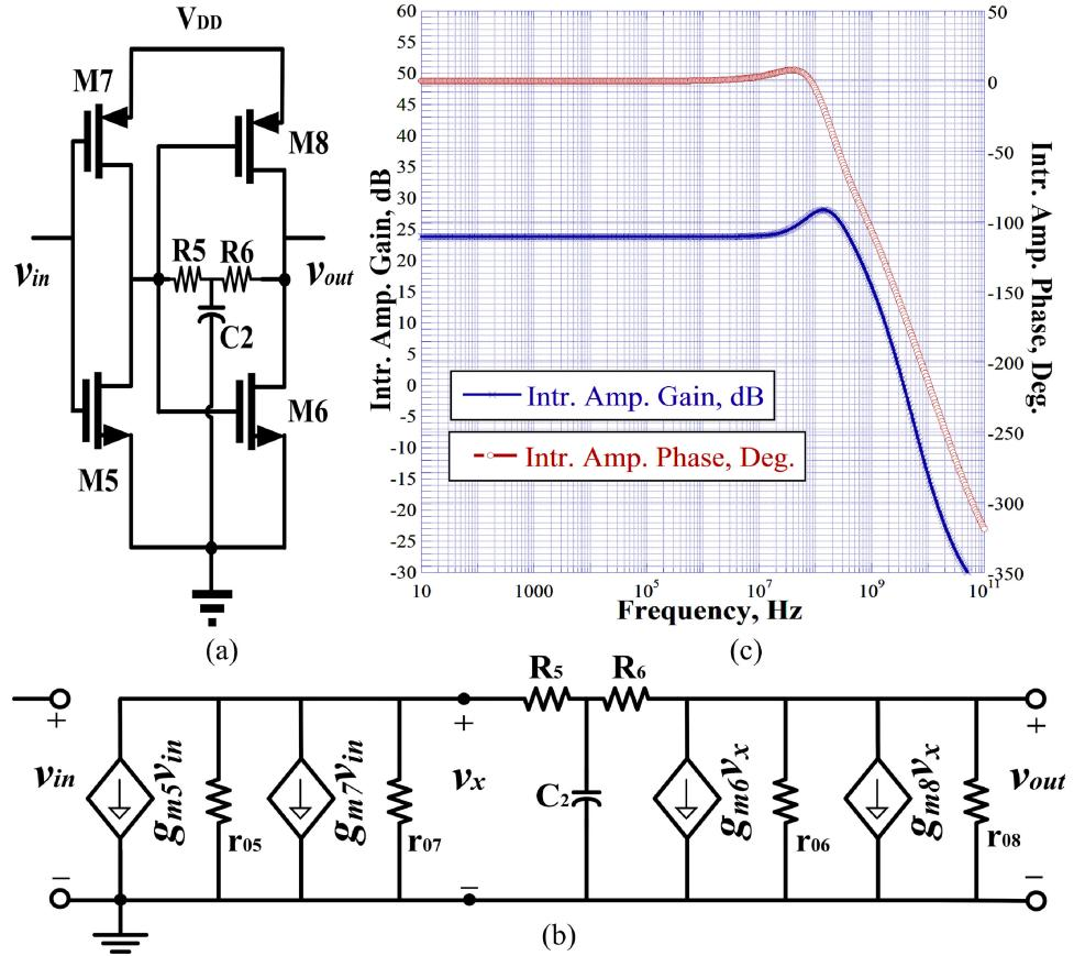
Fig. 3. (a) Intermediate voltage amplifier (b) Its small signal equivalent (c) Gain and phase response.
