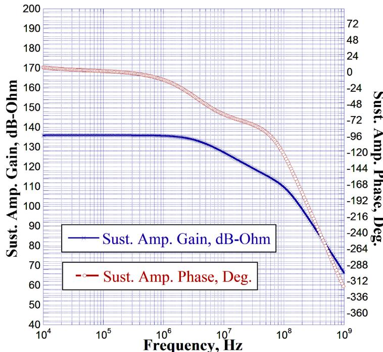
Fig. 5. Bode plot of the complete sustaining amplifier.
