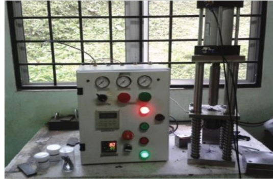
FIGURE 1.—Custom-made vertical metal injection molding machine.
