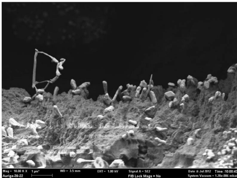
Fig. 2. (a) FESEM image of as-synthesized a-CNTs. (b) FESEM images of Au nanoparticles decorated a-CNTs treated with 10 g/dm 3 AuCl solution.
