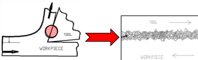
Figure 12. Rolling elements in the tool-chip interface [16]
