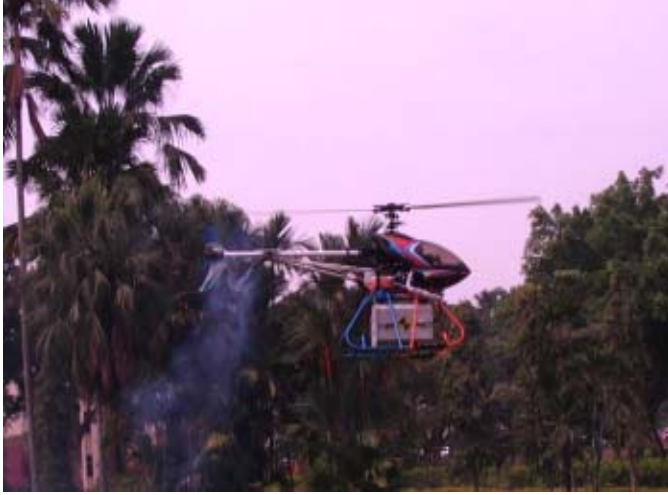
Fig. 2 photograph of Collecting Flight Data for System Identification
