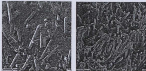
Fig. 8. SEM micrograph taken from tensile fracture surface of composite under dry (left) and wet (right) conditions.
