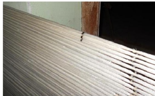
Plate 5: Marking of design with charcoal slurry on silk yarn
